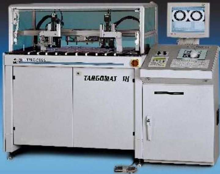
Targomat-IV Post-Etch registration and Layup tooling-hole drilling machine
